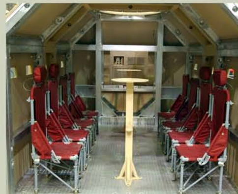
Multiple-Seating Configuration – Facing Inboard
