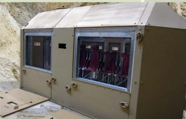
Multiple Egress Hatches and Locations (with push-out side panels removed)
